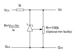
This circuit will allow the reference to be trimmed over a wide range. The device is specified over a  $\pm 5\%$  trim range.
