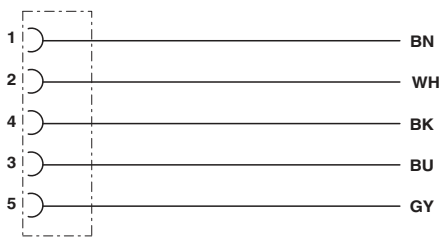
Contact assignment of the M12 socket
