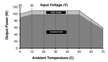
Derating requirements - Derate from 100% load at 50°C to 50% load at 70°C.
