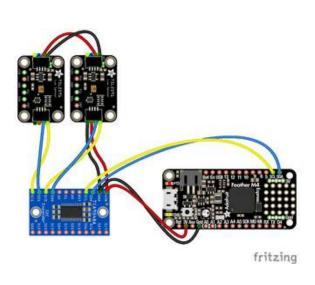
Board 3V to mux VIN (red wire) Board GND to mux GND (black wire) Board SCL to mux SCL (yellow wire) Board SDA to mux SDA (blue wire)
