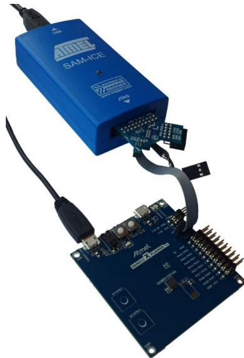
Figure 7-7. SAM-ICE using an Atmel-ICE Adapter
