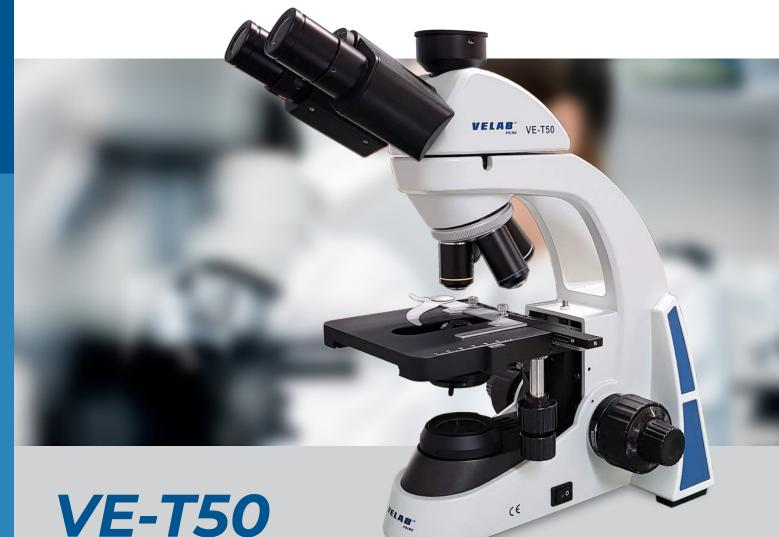
Trinocular biological microscope designed for developing advanced microscopy techniques. Ideal for research, higher education and for diagnostic work in clinical laboratories. Its trinocular head is adaptable to digital devices (not included) for image and video documentation. Its mechanical stage provides fine and smooth movement control, providing precise orientation, a useful feature during histology and cytology tests. The diopter adjustment (on one eyepiece) let you compensate
