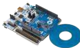
X-NUCLEO-NFC04A1 ST25DV-I2C based Dynamic NFC tag Nucleo expansion board
