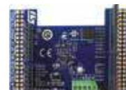
STEVAL-IOD003V1 IO-Link (PHY) device evaluation board based on L6362A with Arduino connectors for STM32 Nucleo
