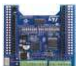
X-NUCLEO-PLC01A1 Industrial input/output expansion board based on VNI8200XP and CLT01-38SQ7 for STM32 Nucleo
