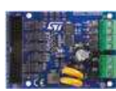
STEVAL-IFP029V1 Industrial digital output expansion board based on ISO8200AQ for STM32 Nucleo
