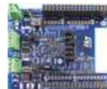
STEVAL-IOM001V1 IO-Link master evaluation board based on L6360 equipped with ST morpho connectors for STM32 Nucleo
