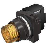
30mm BlackMax, Epoxy Coated Corrosion Resistant Complete Metal Unit Illuminated Indicator Light Transformer type, 600V AC LED Lamp, BA9s Plastic Lens, Amber UL Listed, CSA Certified NEMA 1,3,3R,4,4X,12,13 & Automotive Standards
