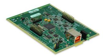
The OEM versions have the same specifications as the standard devices, but come in a board-only form factor with header connectors instead of screw terminals.
