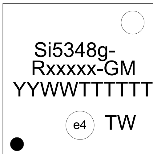
Figure 12.1. Si5348 Top Marking
