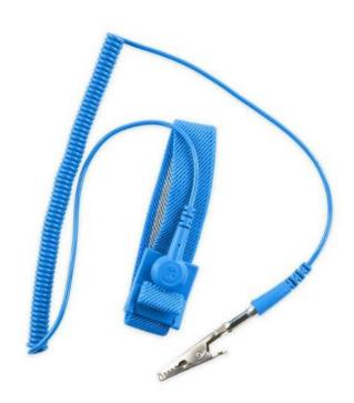
"Rapid static dissipation by a wrist strap ground is required to prevent voltage spikes. Simple movements such as lifting one foot off the floor or raising one arm from a conductive table mat may change body capacitance by as much as 10% to 30%. Uncontrolled, the capacitively created voltage may reach several hundred volts or more."
