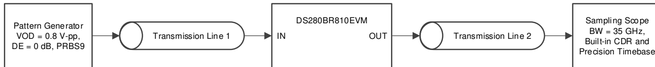
Figure 20. 10 in Rx and 5 in Tx Channel Test Setup
