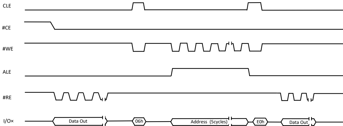
Figure 9-4 Two Plane Random Data Read (06h-E0h) Operation
