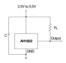
Note: 5. C is for power stabilization and to strengthen the noise immunity, the recommended capacitance is 10nF to 100nF. R<sub>L</sub> is the pull-up resistor, the recommended resistance is 10kΩ to 100kΩ.
