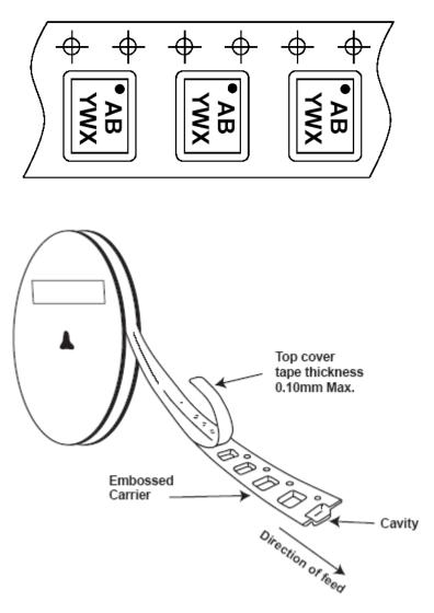
Notes: 10. The taping orientation of the other package type can be found on our website at http://www.diodes.com/datasheets/ap02007.pdf.
