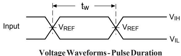
**Voltage Waveforms - Pulse Duration**
