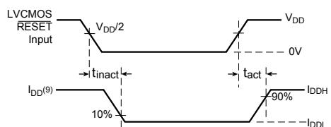
**Voltage and Current Waveforms
