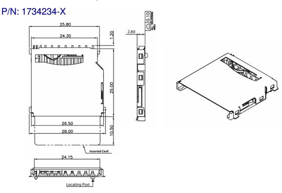
Full Size Connector: Top Mount, Push/Push Insertion/Removal
