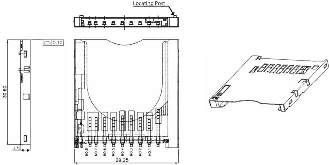
Mini Connector: Bottom Mount, Push/Push Insertion/Removal
