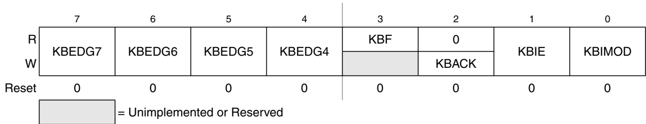
Figure 9-3. KBI x Status and Control Register (KBIXSC)
