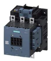
power contactor, AC-3e/AC-3 150 A, 75 kW / 400 V AC (50-60 Hz) / DC Uc: 200-277 V PLC input 24 V DC 3-pole, auxiliary contacts 2 NO + 2 NC drive: electronic main circuit: busbar control and auxiliary circuit: spring-loaded terminal
