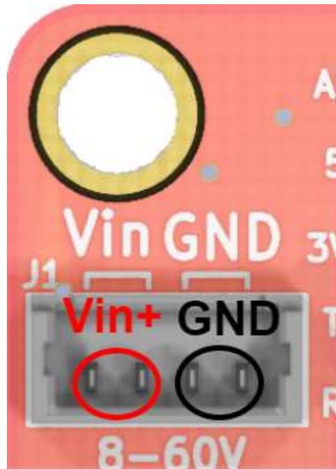
Figure 4: Voltage input header pinout
