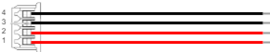
Figure 7: Voltage input cable pinout (red = 5V, black = GND)
