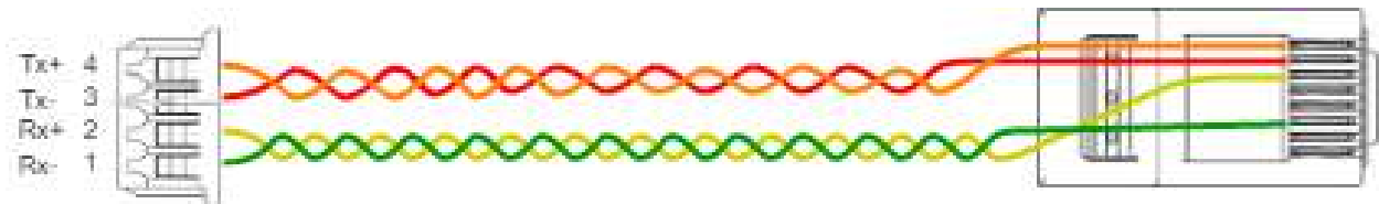
Figure 9: Ethernet cable pinout
