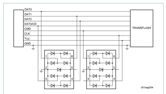
Fig 6. Typical application for universal microSD/TransFlash and SD memory card ESD protection
