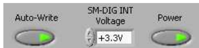
Figure 18. Auto-Write, Power Button, and Voltage Control
