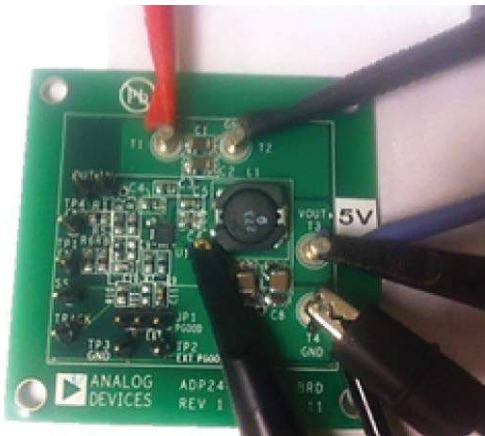
Figure 4. Switch Node Measurement
