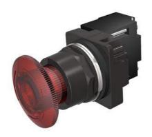
30mm BlackMax, Epoxy Coated Corrosion Resistant Metal Operator, Round Illuminated Twist-to-Release Transformer type, 600V AC Incandescent Lamp Mushroom Head Cap Small 1.79" (45 mm) Plastic Cap, Red 2 Position Maintained, Twist-to-Release UL Listed, CSA Certified NEMA 1,3,3R,4,4X,12,13 & Automotive Standards
