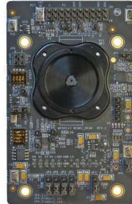
Figure 1. MT9V117 Evaluation Board
