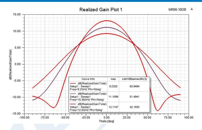
Click the following link (or enter part number in "SEARCH" on website) to obtain additional part information including price, inventory and certifications: WR-90 Standard Gain Horn with 10 dBi gain, End Launch SMA Female connector PEWAN090-10ELSF
