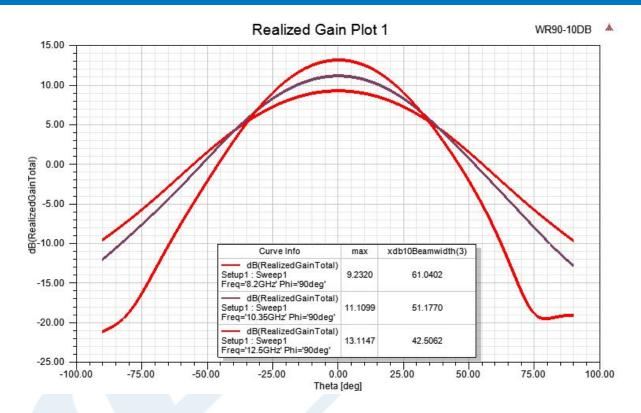
WR-90 Standard Gain Horn with 10 dBi gain, End Launch SMA Female connector from Pasternack Enterprises has same day shipment for domestic and International orders. Our RF, microwave and millimeter wave products maintain a 99.4% availability and are part of the broadest selection in the industry.
