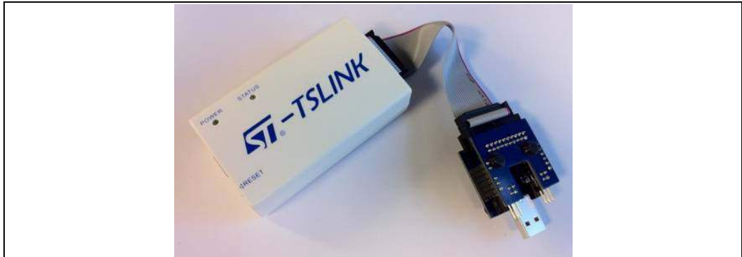
Figure 11. MB973/MB972 board assembly connected to ST-TSLINK dongle
