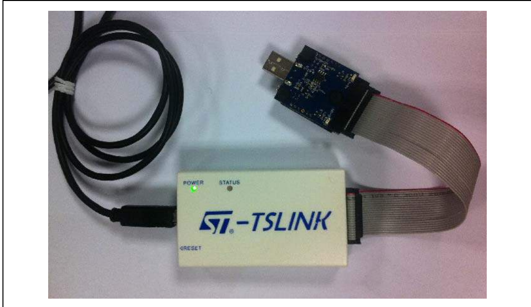
Figure 5. ST-TSLINK programming dongle
