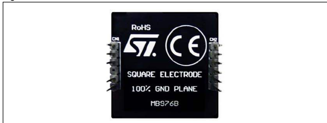
Figure 6. MB976 electrode board
