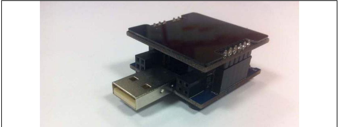
Figure 8. MB976 electrode board connected to MB972 controller board
