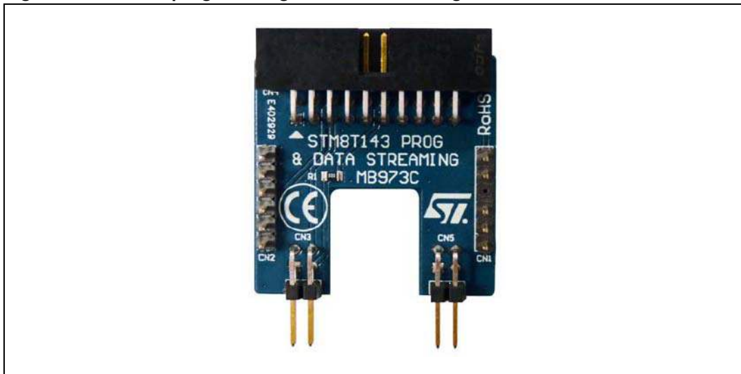
Figure 4. MB973 programming and data streaming board
