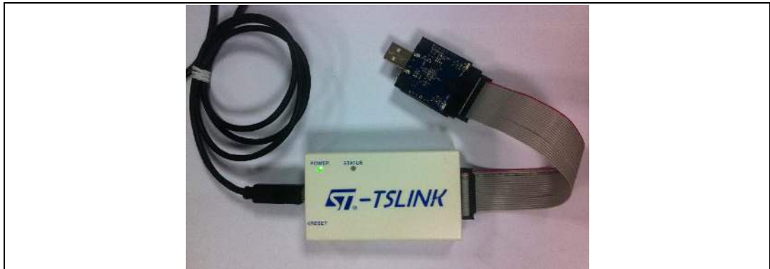
Figure 12. MB973/MB972 board assembly and ST-TSLINK dongle with USB connector
