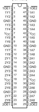
To ensure the high-impedance state during power up or power down,  $\overline{OE}$  should be tied to  $V_{CC}$  through a pullup resistor; the minimum value of the resistor is determined by the current-sinking capability of the driver.
