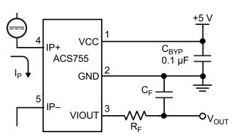
Application 1. The ACS755 outputs an analog signal, V<sub>OUT</sub>. that varies linearly with the unidirectional DC primary sampled current, I<sub>P</sub>, within the range specified. C<sub>F</sub> is recommended for noise management, with values that depend on the application.
