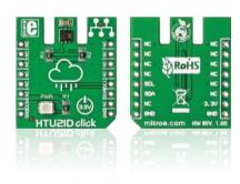
HTU21D click<sup>™</sup> carries a high-precision, easy-to-use relative humidity sensor with temperature output. The sensor is plug and play, requiring no calibration to use. The measurement range of HTU21D click<sup>™</sup> is from 0 to 100 percents of relative humidity, and -40 to +125 degrees of Celsius. The board communicates with the target microcontroller through mikroBUS<sup>™</sup> I2C lines: SCL and SDA (data). It uses a 3.3V power supply only.
