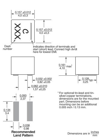
Packaging 500/7" reel; 2000/13" reel Plastic tape: 12 mm wide, 0.30 mm thick, 8 mm pocket spacing, 4.27 mm pocket depth
