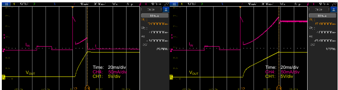
Figure 51. Si3406-ISO-FB EVB, 12 V, Class 2 Output Voltage Soft-Start at Low Load (Left) and Heavy Load (Right) Conditions
