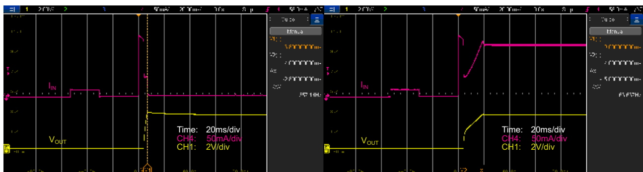
Figure 13. Si3406-ISO-FB EVB, 3.3 V, Class 2 Output Voltage Soft-Start at Low Load (Left) and Heavy Load (Right) Conditions
