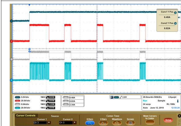
Figure 8-9. ITRIP Across TOFF and Load Current
