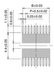
Note: Shaded area should be free of any conductive traces.
