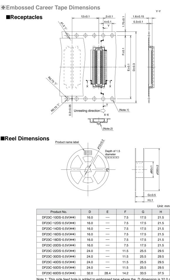
Note 1: This side feed hole is added to embossed tape where the D dimension is 32.0 min. wide. Note 2: (53) packaging code embossed tape is without the bottom surface protrusion. The product information in this catalog is for reference only. Please request the Engineering Drawing for the most current and accurate design information. All non-RoHS products have been discontinued, or will be discontinued soon. Please check the products style in the dissemble di
