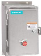
Non-reversing motor starter Size 0 Three phase full voltage Solid-state overload relay OLRelay amp range 0.25-1A 550/575-600 50/60HZ coil Combination type Water/dust tight non-corrosive
