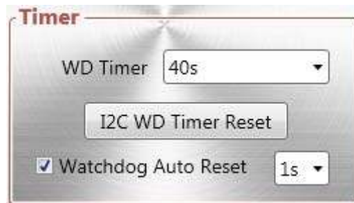
Figure 8: Setting the Watchdog Timer Limit
