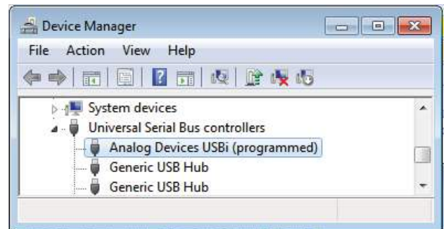
Figure 9. Confirming Driver Installation Using the Device Manager
