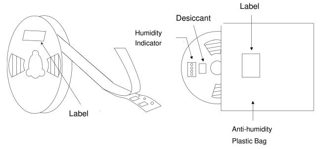
Tape and reel must be sealed with the anti-humidity plastic bag. The pag contains the desiccant and the humidity inductor.
