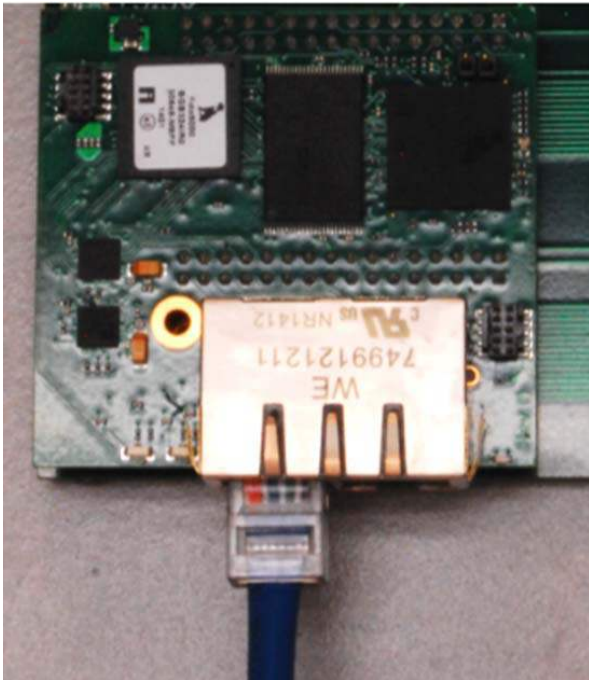
Figure 6. Ethernet Cable Connection
