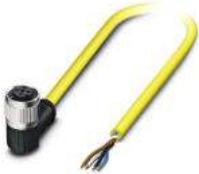
Sensor/Actuator cable, 4-position, TPE, yellow RAL 1021, free cable end, on Socket angled M12 SPEEDCON, A-coded, Cable length: 2 m
