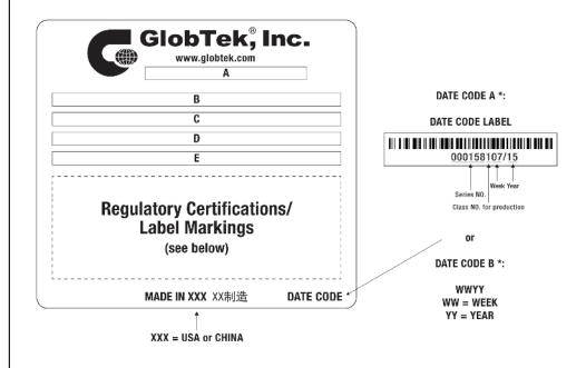
A=PoE, Passive Power Injector B=P/N: (料号) GT-96300-3648-T2-PP C=Model (型号) GT-96300-3648-T2-PP D=Input (输入)100-240V~, 50-60 Hz, 1.0A E=Output (输出)48.0 V == 0.75 A, 36.00W
