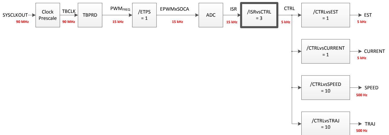
Figure 9-15. Software Execution Clock Tree for ISR Waveforms
