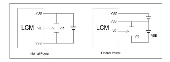
$V_{\text{DD}^{\sim}}V_{0}\text{: LCD}$  Driving voltage
