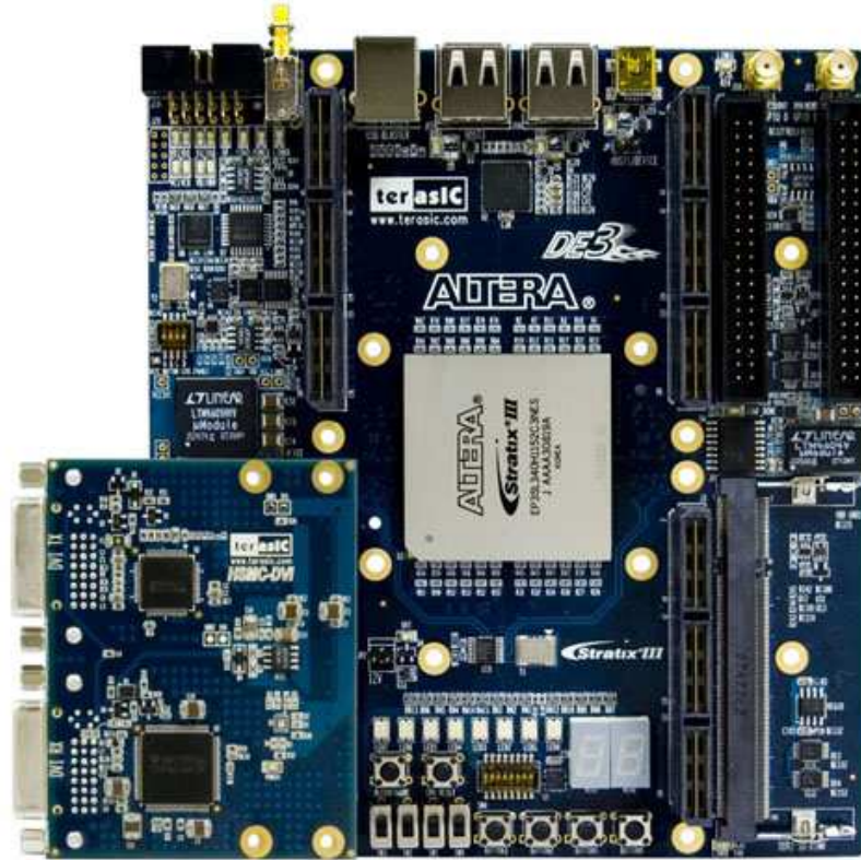
Figure 1.2.1 The HSMC-DVI board connects with DE3
