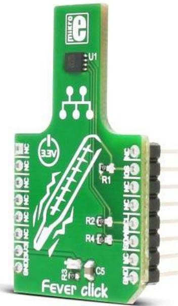
**Fever click** measures your body temperature with the accuracy of 0.1°C (37°C to 39°C). The click carries MAX30205 human body temperature sensor. Fever click is designed to work on a 3.3V power supply. It communicates with the target MCU over I2C interface.
