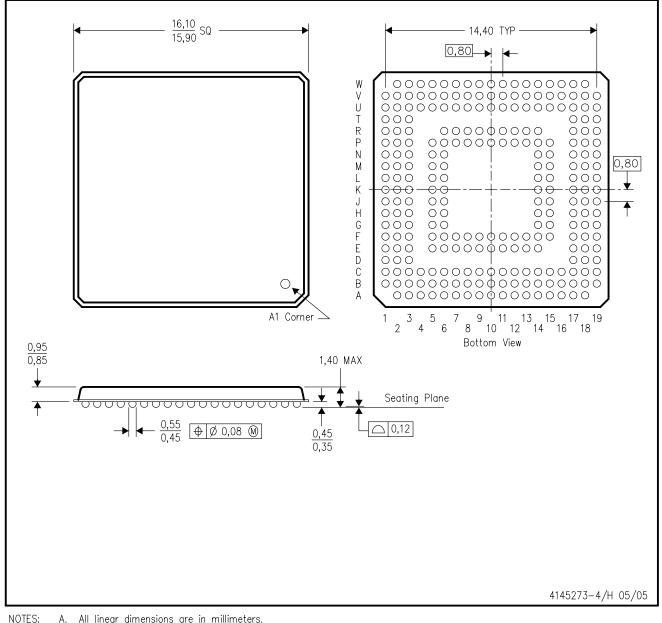
A. All linear dimensions are in millimeters.
