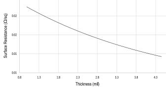
Surface Resistance by Paint Thickness
