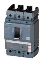
circuit breaker 3VA5 UL frame 250 breaking capacity class H 65kA @ 480V 3-pole, line protection TM210, FTFM, In=90A overload protection Ir=90A fixed short-circuit protection Ii=10 x In UL 489 SB (naval), 50 °C without connection
