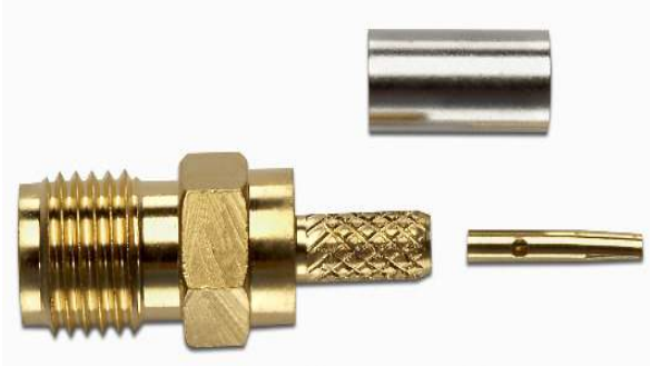
Model 72954 SMA JACK STRAIGHT CRIMP, RG174, 188, 316
