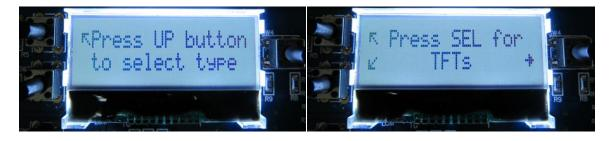
9. The NHDev display will show the first part number model in the selected category. Pressing UP and DOWN buttons will cycle through the available part number models that NHDev is programmed to demonstrate. When the desired part number model is reached, stop pressing buttons.
