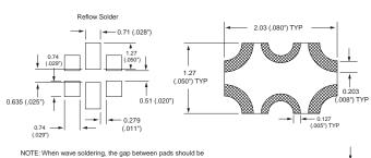
NOTE: When wave soldering, the gap between pads should be covered with photo-imageable solder mask to prevent bridging between terminations under the component. Also the spacing between the ground contacts should be increased from .635mm (.025") to .889 (.035").
